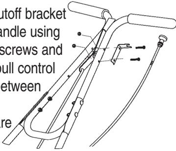
**8** Attach lever bracket to the handle using the two 1 1/4" Phillips screws and two lock nuts. Be sure that the bracket is aligned as shown in the diagram.
