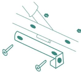
Place the spring on the end of the deflector rod with the formed tabs as shown. Insert end of rod through the hole in the deflector bracket. Slide the rubber cap onto end of the rod. Note: move end of deflector rod to the up position (deflector is up).
